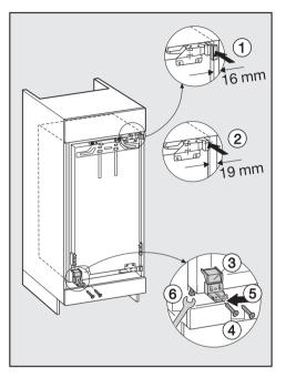
Depending on the thickness of the appliance housing unit walls, push the appliance into the niche until
